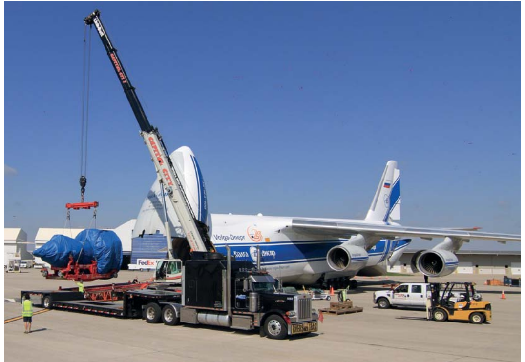
Loading a GE GE9X aero engine on a Volga-Dnepr An-124 freighter
