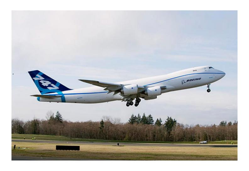
The 747-8 Freighter is the new, high-capacity 747 that will give cargo operators the lowest operating costs and best economics of any freighter. The airplane is 250 feet, 2 inches (76.3 m) long, which is 18 feet, 4 inches (5.6 m) longer than the 747-400 Freighter.
