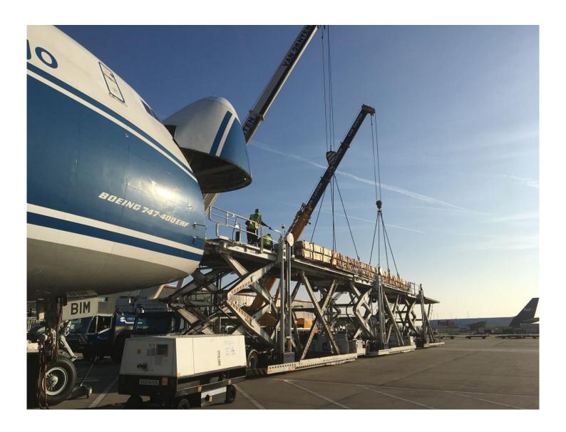
Eight crates weighing around 20,000 kg and measuring 2200x50x50cm were loaded through the 747's nose-swing door in Amsterdam, with the help of two loading cranes, in preparation for the delivery to
